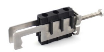
KwikClamp™ Hanger for 1/4 in superflexible coaxial cable, triple stack; includes hardware
