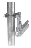
Middle Downtilt Mounting Kit for Long Antennas for 2.4 - 4.5 in (60 - 115 mm) OD round members. Kit contains one scissor bracket set.
