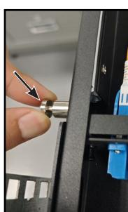
**3** Pull outward on the top cover clips to unlock, then remove the cover. For MPO cassettes installations slide the cassettes into place and lock them on the panel by pressing in the clips.
